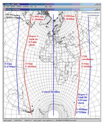
Great care has been taken, to eliminate loss of precision, leading to, e.g., the implementation of an *extended range transverse mercator* code, remaining accurate (and roundtrip-consistent) at the 0.03 mm level, even at distances 7500 km from the central meridian (figure above).
