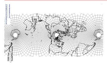
The figure to the left shows how the extended range transverse mercator implementation may even be (mis)used to produce (almost) global maps, while remaining consistent and accurate. Such unorthodox tricks may actually prove useful in rare cases. It is, however, included here primarily as a curiosity.
